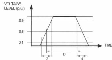
Figure 1: Test waveform
